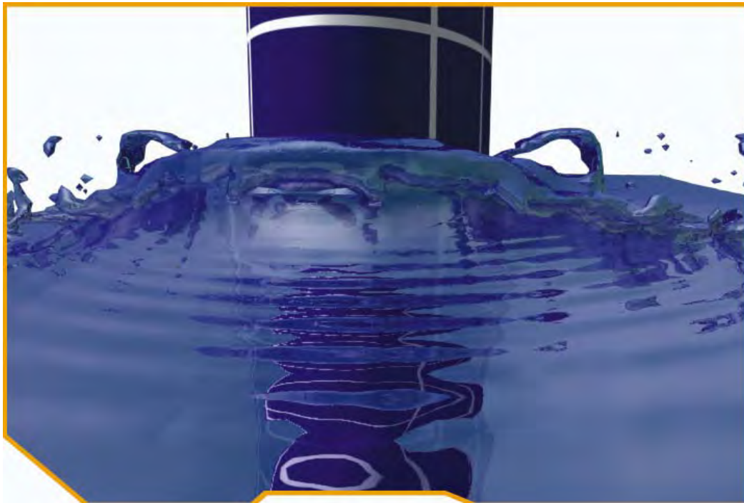
Large-eddy simulation of steep breaking waves and thin spray sheets around a ship
